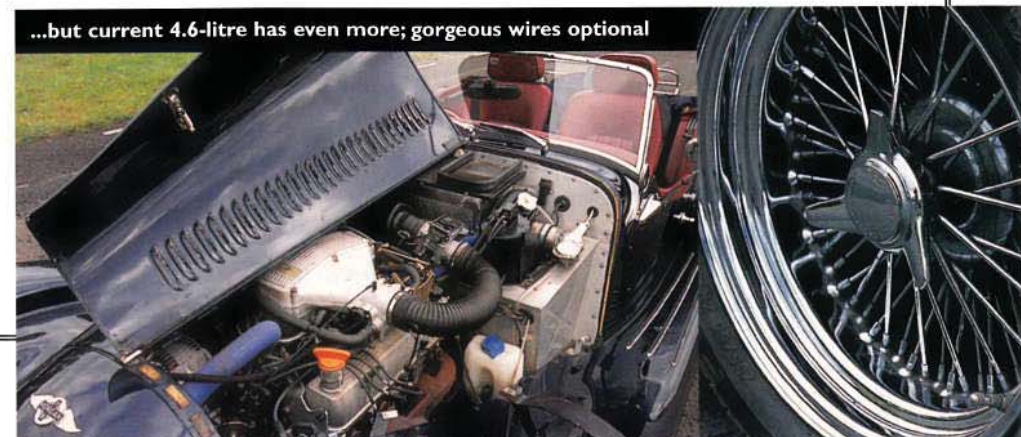
Fuel-system change to injected unit in '94 boosted torque again
