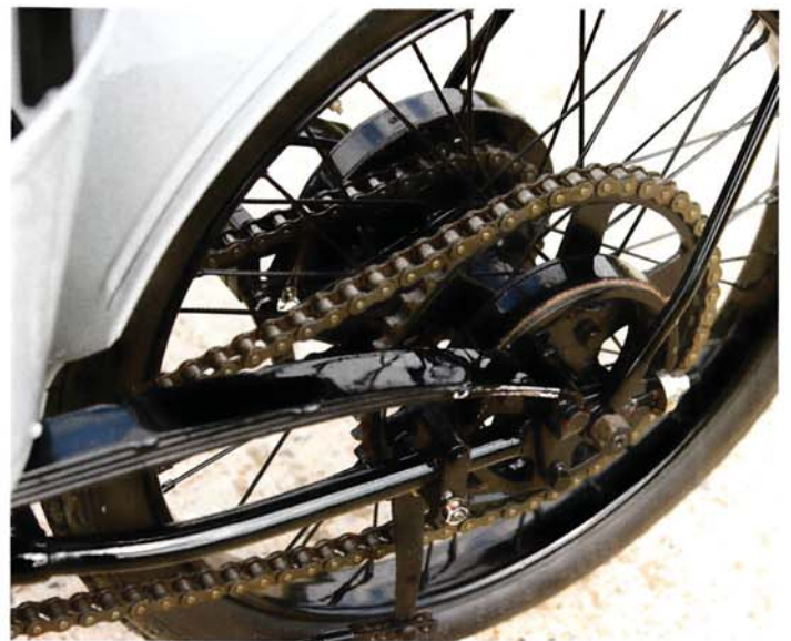
Clockwise, from above: rear fork with twin gears, hand and foot brakes plus reversed springs; manual oil system with plunger and tap; spindly sliding-pillar suspension, gas lighting canister and pepper-pot exhaust
