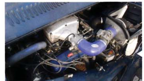
John Eales motor has an aluminium rad and oil catch tank
