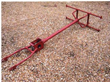
Clockwise, from above: complete chassis with backbone torque tube; body style was planned in timber; Walsh adapts to sensitive tiller steering
